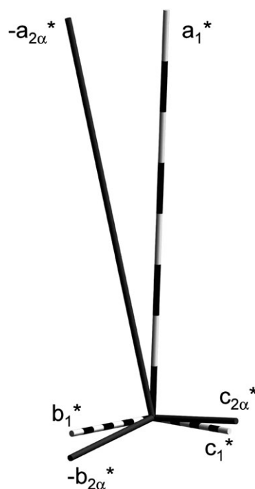
Fig. 1 Reciprocal unit cells of the reactant (dashed black and white) and product crystals (dark grey).
